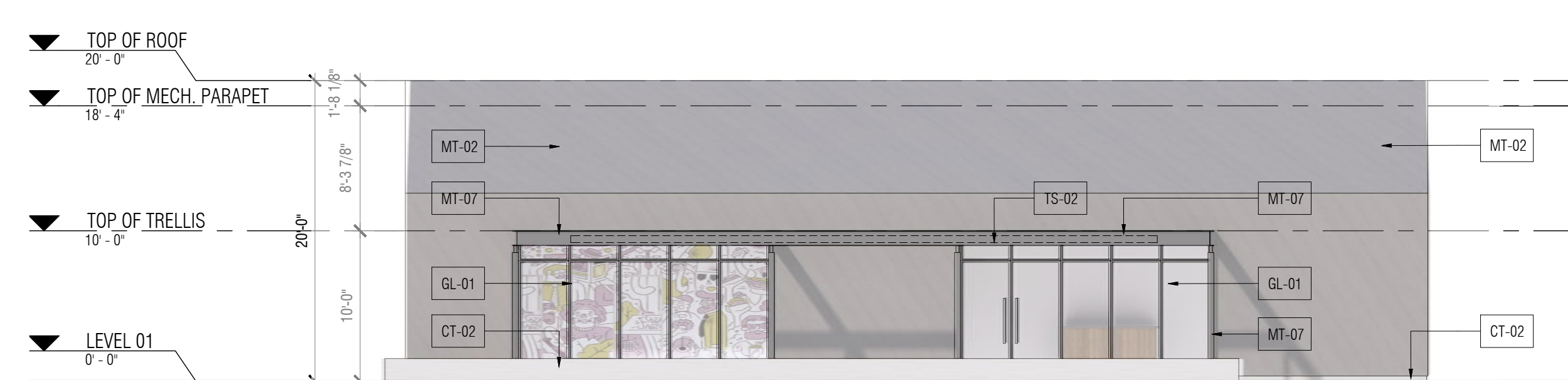
EXTERIOR ELEVATIONS - BUILDING C FRONT SCALE: 1/8" = 1'-0" 4
